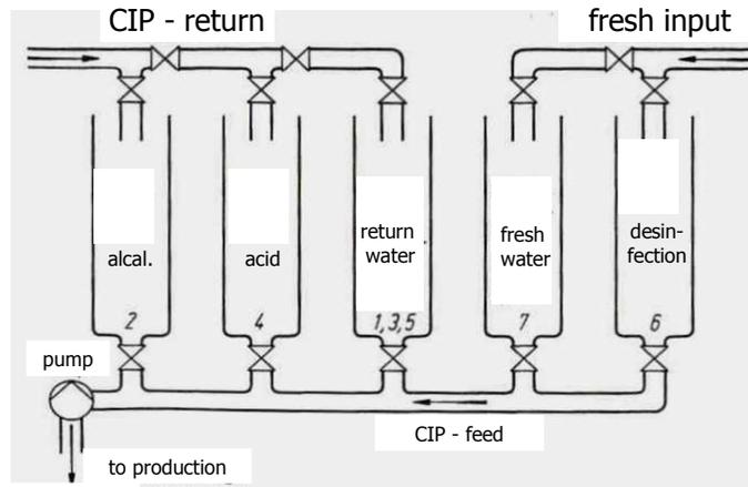
Figure 5: Reusing rinsing water for pre-washing
