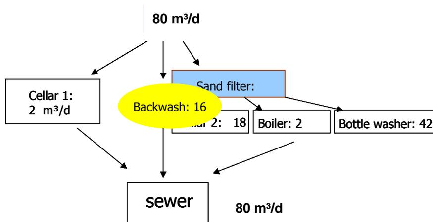
Figure 2: Flowchart for a winery including backwashing
