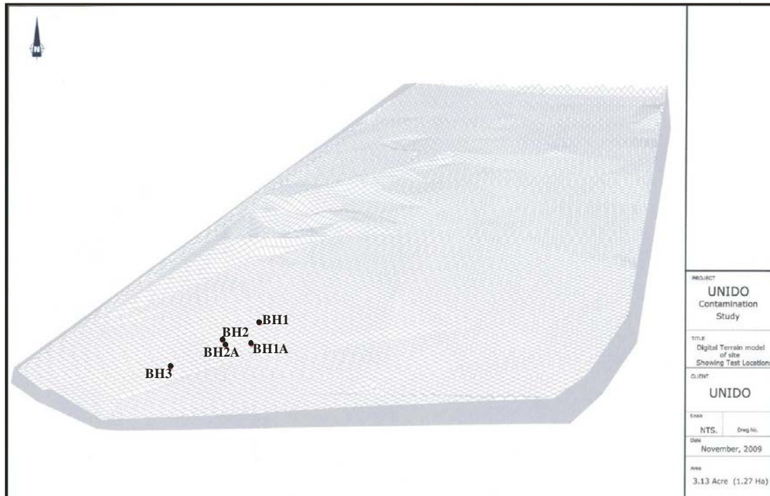
Figure G3.2 Digital terrain model of ECG station G showing locations selected for drilling
