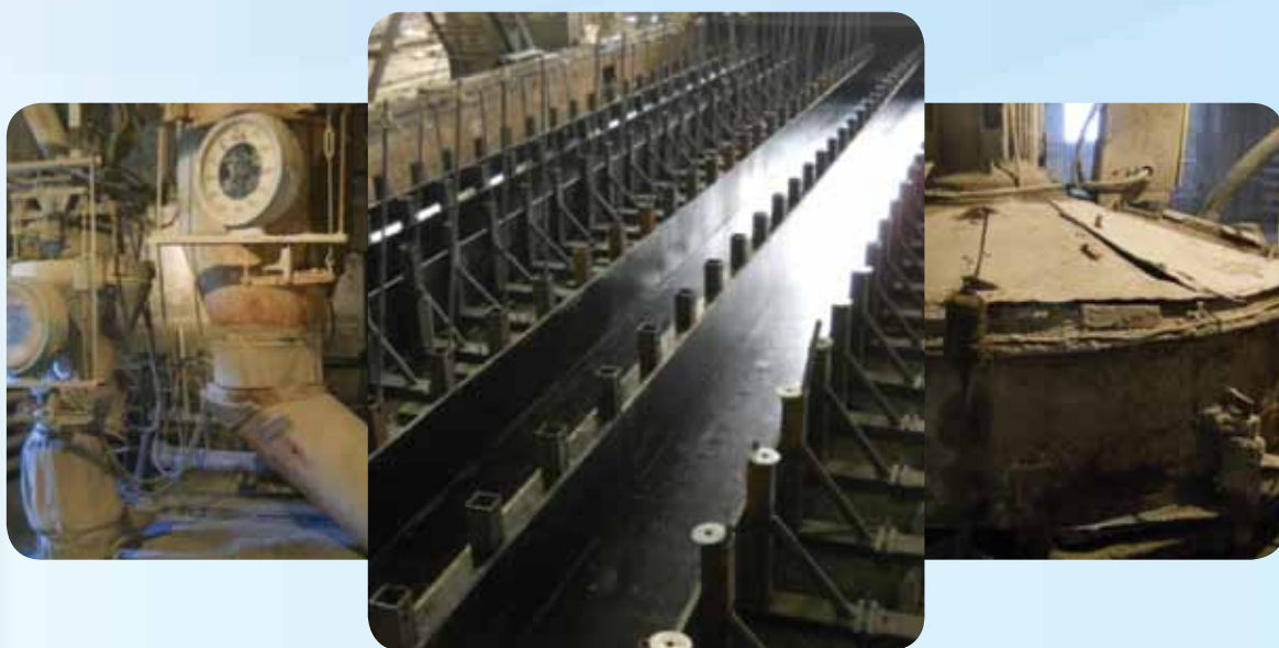
Picture 1: Dosing system, mixing machine and casting mold
